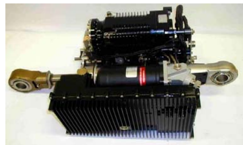
Figure 1: A380 EHA Aileron actuator
