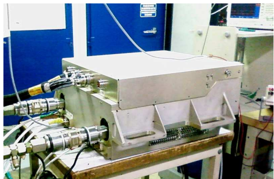
fig.4 - power converter during TAES tests
